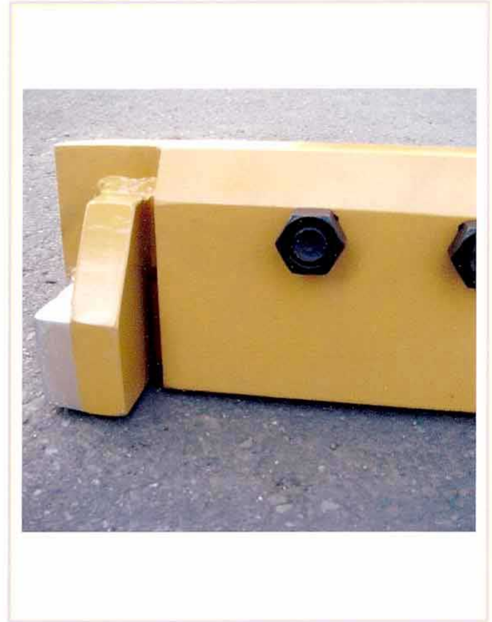
(Above): View Showing (MAG/500) x (1") Thick Rear Support Bar with Castings and (3/8") Clearance from Outside Edge of (I.C.E.) Top Beveled Grader Blade. This is the Standard Clearance.
